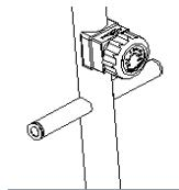
The ALFA2 training Bike is equipped in manual tension regulation. The levels of regulation are designated from “-“ to “+”. Level “-“ is the easiest. Level “+“ is the hardest. It is possible to adjust the level of tension according to the user's need and training plan.
