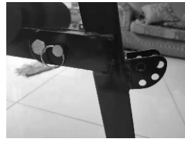
Step 3: open the main frame and position it with bolts
