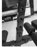
Step 5: pass the tube through the side plate and clamp it with knob
